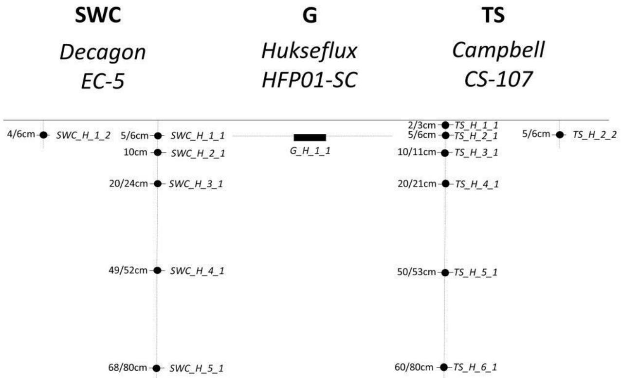
Figure 9: Set-up of the five soil plots (H = 1 to 5). SWC = volumetric soil water content, G = soil heat flux density, TS = soil temperature. X/Ycm indicates per sensor the variation in installation depth between the five plots.
